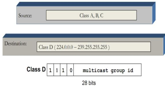
Fig 1: Data packet format for Multicast Routing
